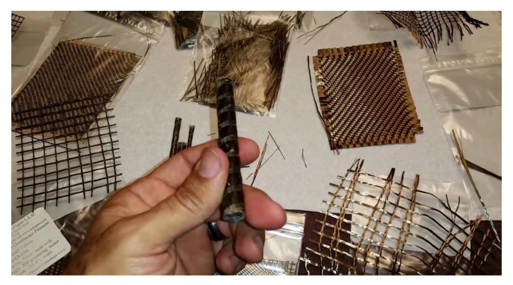
Basalt is almost the same as glass. You melt it and then spin it into fibre the same as fibreglass
